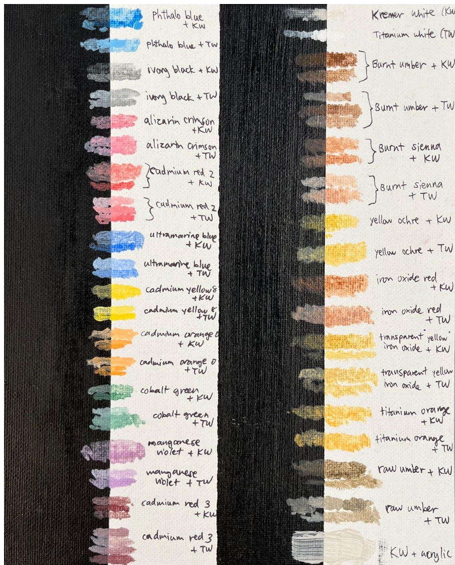
Figure 13. Panel of painted swatches of Kremer White, titanium white, and both whites combined with common inpainting colors.
